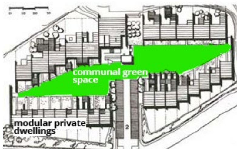
Denmark's Sættedammen site plan features a communal green space in the centre, bordered by two rows of private dwellings, built using modular designs to allow interior walls to move according to living needs. Source: Adapted from Schemata Workshop
