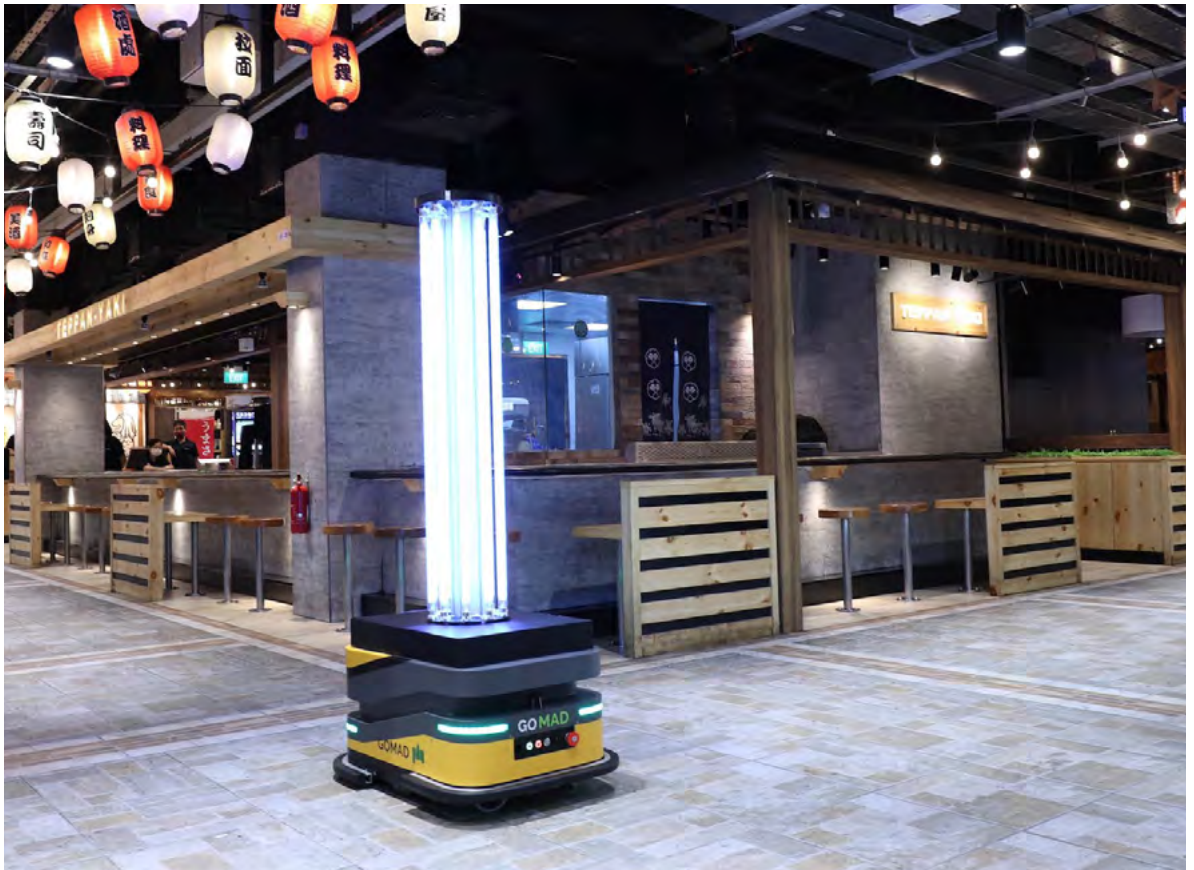
Fig 15. The Sunburst UV Bot, built with a lamp module emitting ultraviolet-C light, conducting disinfection at a shopping centre. Image courtesy of PBA Group.
